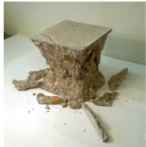
*Fig. 10. Concrete cube specimen after compression test*
