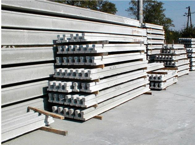
Fig. 23. Beams of type “EE” after manufacture
